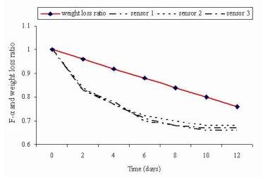
**Figure 2**. F- $\alpha$  and weight loss (expressed in proportion to the initial value) in Flame grapes over a period of time. The estimated weight loss value is a mean of three groups of grapes.
